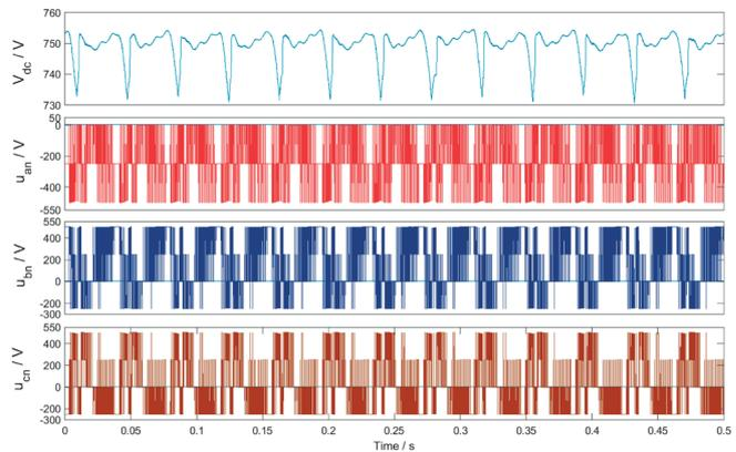
(e) DC bus voltage and inverter phase voltages for  $S_4, S_6$  dual-tube-fault
