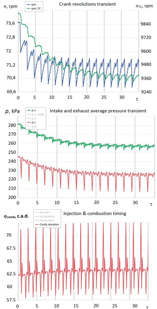
Fig. 5. Results for transient engine operation under a fuel injection irregularity
