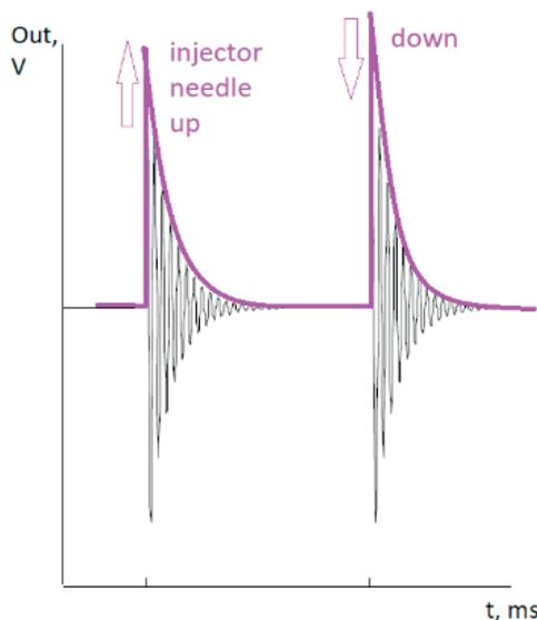
Fig. 2. Amplitude demodulation of high-frequency injector signals [18]
