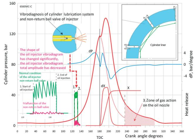
Fig. 7. Vibration diagram for the cylinder lubrication injector, combined with a P(deg) diagram
