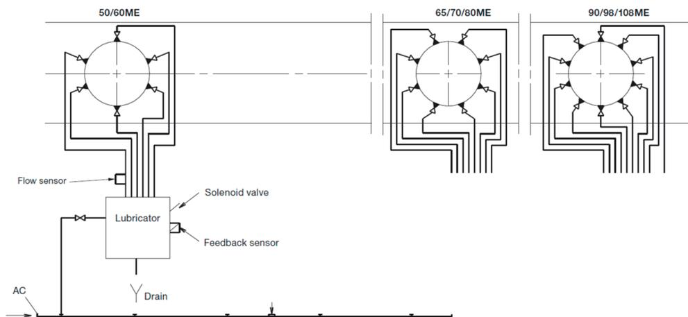
Fig. 8. Cylinder lubricator system for ME engines [23]
