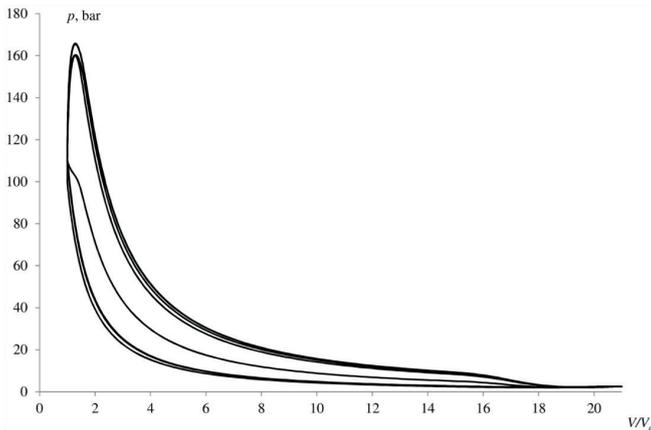
Fig. 6. Cycle variations under irregular fuel injection conditions
