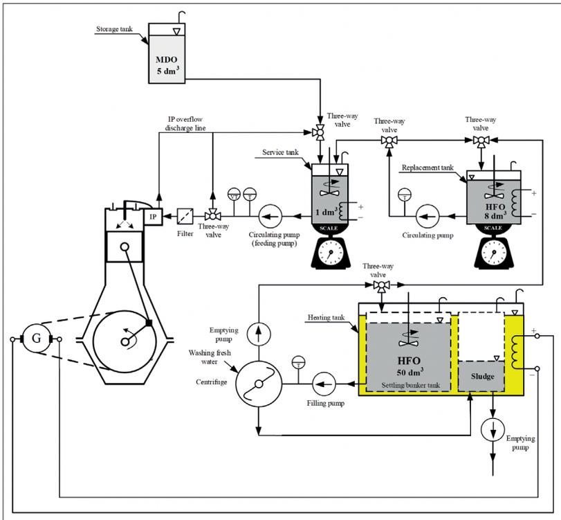
Fig. 1. Schematic diagram of the fuel feed system of the laboratory Farymann Diesel engine D10 type: MDO - (Marine Diesel Oil) marine distillate fuel; HFO - (Heavy Fuel Oil) marine residual fuel; IP - injection pump; VT - viscometer; T - thermometer
