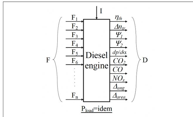
Fig. 7. Physical model of the fuel usability in a single-cylinder diesel engine: F - the set of the considered marine fuels, D - the set of diagnostic parameters, I - interference, Pload - engine output (net) power
