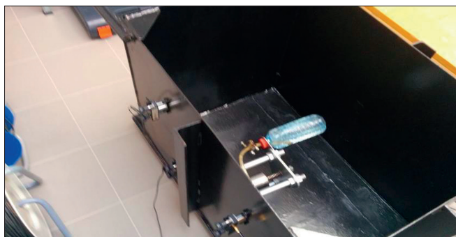
Fig. 4. Corrosion test tank with the KE-2 corrosion tester attached and the VS75-V and VS150 RIC acoustic sensors installed.
