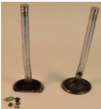
Fig. 5. View of studied damaged valves.
