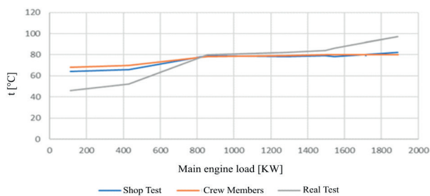
Fig. 13. Dependence of cooling water temperature on the main engine load: blue line - measurement from engine shop tests; red line - measurement taken by the crew; grey line - measurement taken for the sake of the case study.
