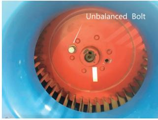
Fig. 1. Blower imbalance fault setting
