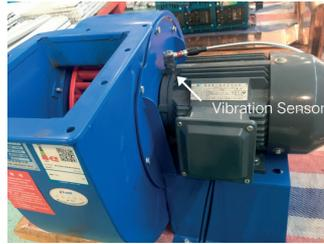
Fig. 2. Blower test bench
