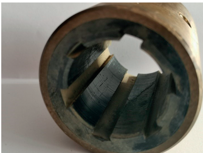
Fig. 5. The PTFE sliding bush (B)
