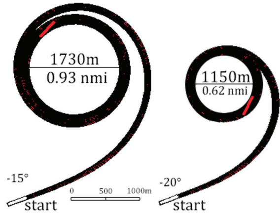
Fig. 4. Simulation results of Esso Norway II turning circle for two rudder deflections
