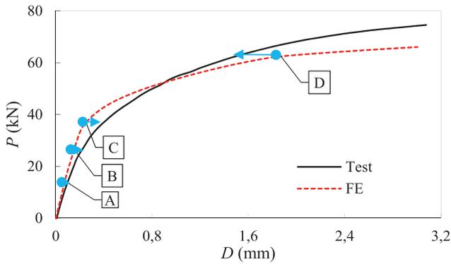
Fig. 7. Force versus displacement of the test sample
