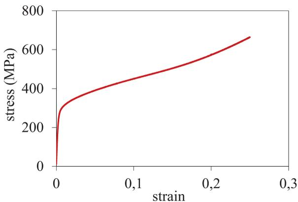
(b) Tensile test results
