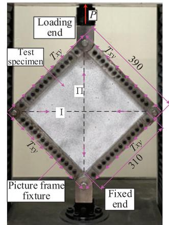
Fig. 4. Test setup of specimen and frame fixture
