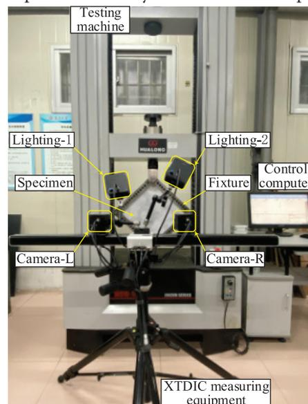
Fig. 5. Shear buckling test of the ship's thin plate
