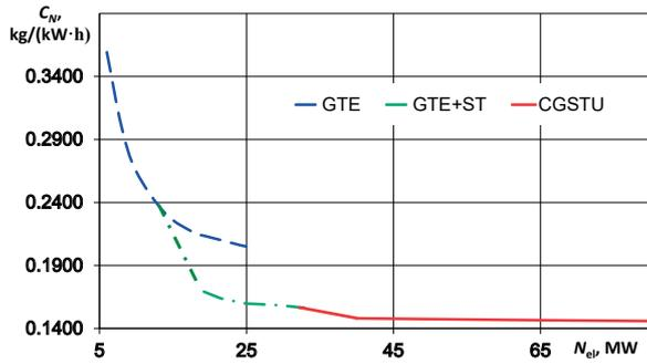
Fig. 10. Dependences of specific fuel consumption on the CGSTU power.
