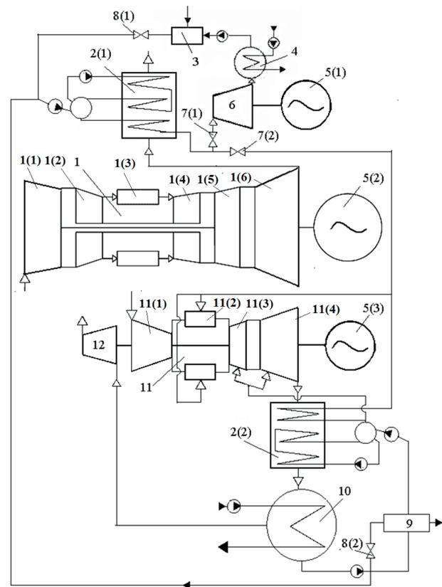
Fig. 1. Thermal diagram of the combined gas-steam turbine unit of a hybrid cycle: 1 - GTE UGT25000; 1(1) - LPC; 1(2) - HPC; 1(3) - CC; 1(4) - HPT; 1(5) - LPT; 1(6) - GT; 2(1), 2(2) - HRSG; 3 - boiler water tank; 4 - steam condenser; 5(1), 5(2), 5(3) - electric generators; 6 - ST; 7(1), 7(2) - steam valves; 8(1), 8(2) - water valves; 9 - water treatment unit; 10 - gas-steam condenser; 11 - SIGT; 11(1) - C; 11(2) - CC; 11(3) - CDT; 11(4) - GT; 12 - exhauster.
