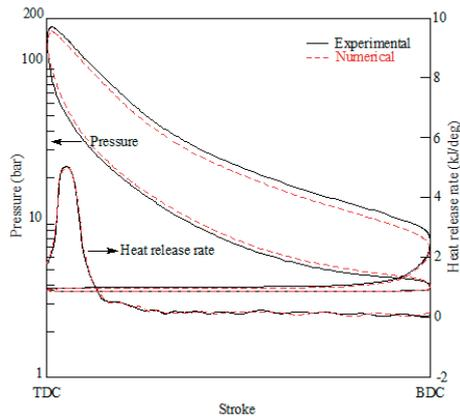
Fig. 2. In-cylinder pressure at 100% load
