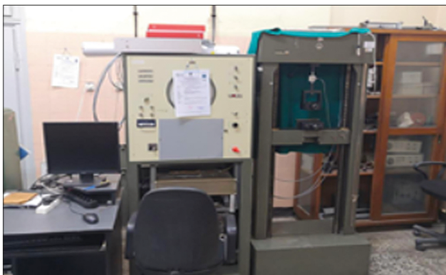
Fig. 7. Laboratory station for measuring Young’s modulus
