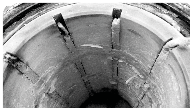
Fig. 1. Elastomer bush melted during the laboratory test. Test conditions: load: 0.2 MPa, speed 10 rev/s, water flow 0 L/min.
