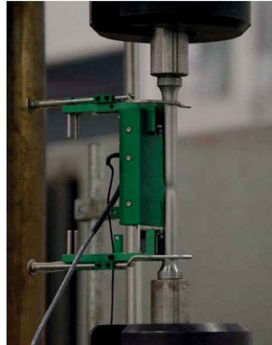
Fig. 2. Specimen during tension test. Moment of necking can be observed
