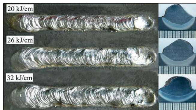
Fig. 4. Bead-on-plate welds and cross-section of welded joints
