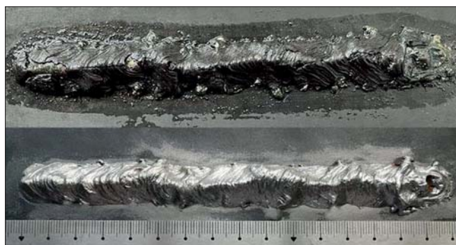
Fig. 2. Surface weld appearance before/after slag removal
