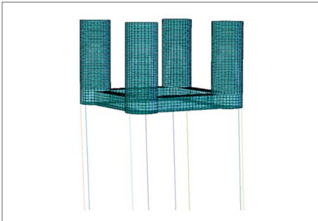
Fig. 11. The mesh of tension leg platform
