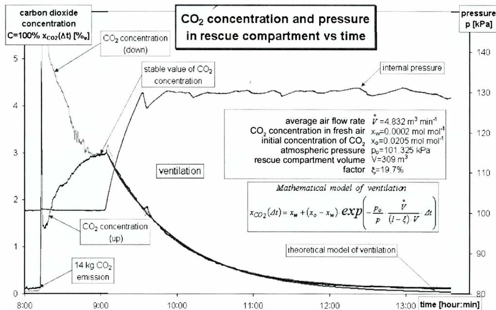
Fig.3. Results of measurements and calculations of  $\text{CO}_2$  concentration in ventilated DISSUB's compartment
