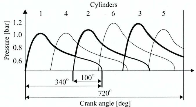
Fig.3. Course of exhaust gas changeable pressure in outlet passages of 6AL 20/24 SULZER diesel engine before the turbine
