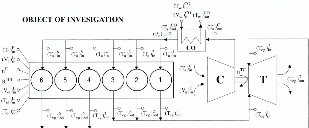
Fig.2. Scheme of the turbocharging system of 6AL20/24 SULZER diesel engine
