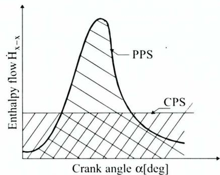
Fig.1. Schematic diagram of change courses of the delivered enthalpy flow  $\dot{H}_{x-x}$  (at the same exhaust gas amount in the outlet section of the radial-flow turbine guide vanes of the turbine-blower) for the two turbocharging systems : PPS - pulsatory pressure system ; CPS - constant pressure system
