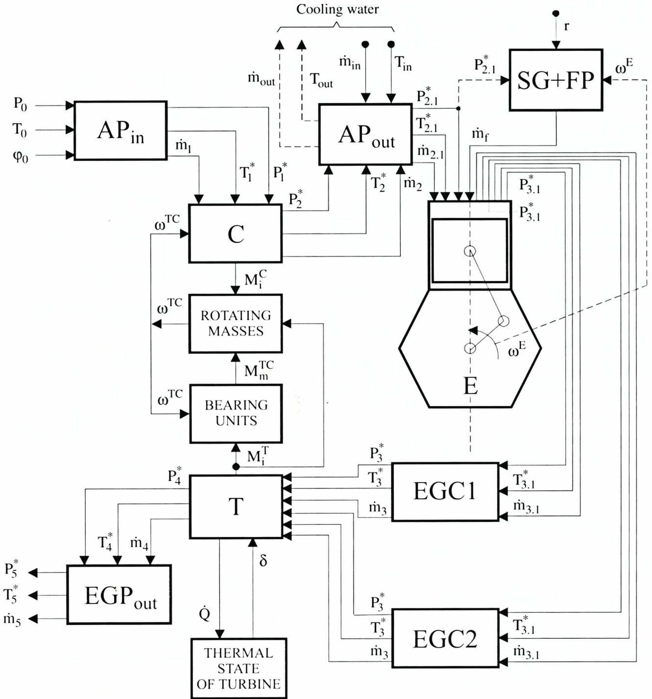
Fig.4. Schematic model of physical process of working medium flow through the air-charging system of the considered engine
