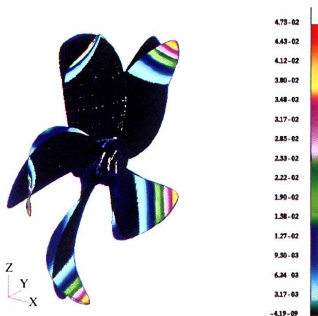
Fig.2. 1 st natural vibration mode of the complete propeller (Case 3)
