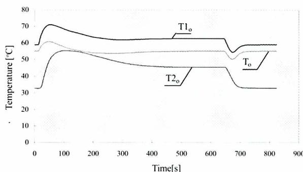
**Fig. 11.** Course of temperature changes versus time within the lubricating oil cooling system (LOI) for a signal given from the ship motion system and the conditions : sea-water temperature of 30 deg C sea-water temperature control system not operating
