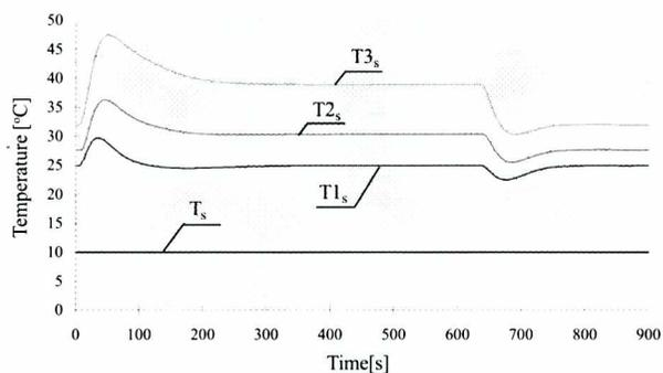
**Fig. 12.** Course of temperature changes versus time within the sea-water cooling system (SWI) for a signal given from the ship motion system and the conditions : sea-water temperature of 10 deg C sea-water temperature control system under operation
