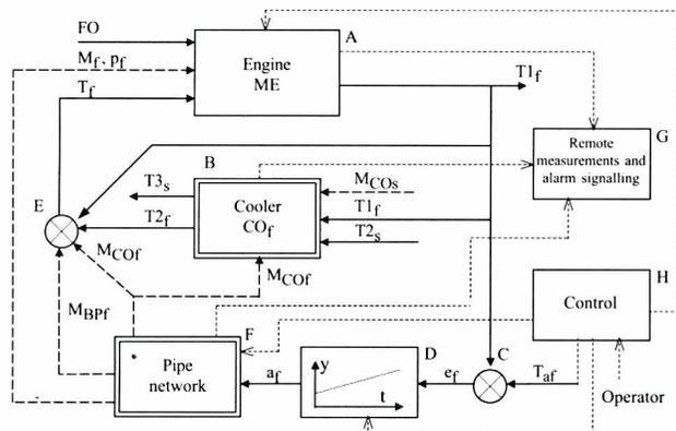
Fig.5. Model scheme of a typical fresh-water cooling system of the main engine
