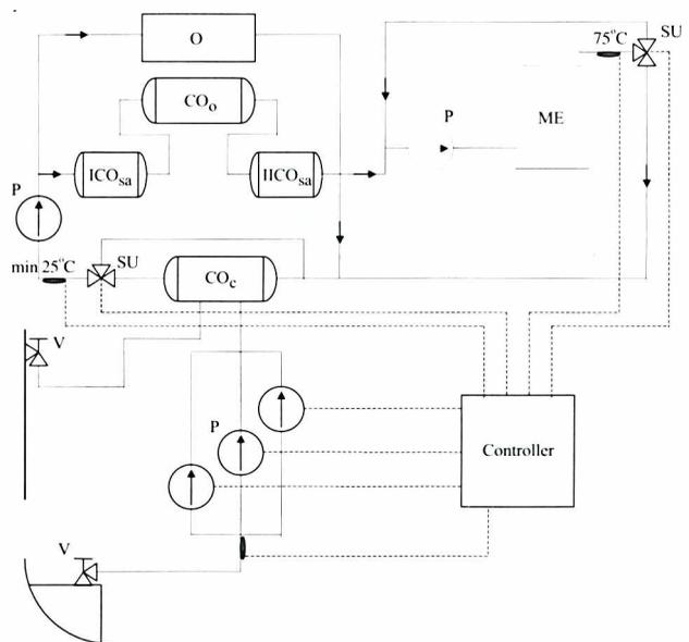
**Fig.3.** Schematic diagram of the central cooling system controlled by the Engard system. **Notation :** COc – central cooler, COo – lubricating oil cooler,
