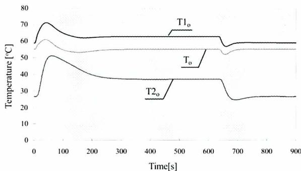
**Fig. 10.** Course of temperature changes versus time within the lubricating oil cooling system (LOI) for a signal given from the ship motion system and the conditions : sea-water temperature of 10 deg C sea-water temperature control system under operation
