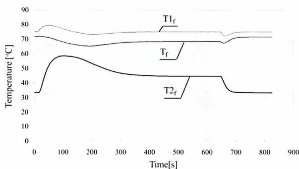
**Fig. 9.** Course of temperature changes versus time within the fresh-water cooling system (FWI) for a signal given from the ship motion system and the conditions : sea-water temperature of 30 deg C sea-water temperature control system not operating
