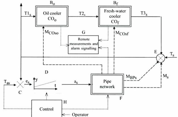
Fig.7. Model scheme of the sea-water cooling system of the main engine
