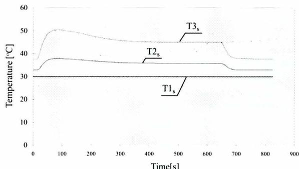
**Fig. 13.** Course of temperature changes versus time within the sea-water cooling system (SWI) for a signal given from the ship motion system and the conditions : sea-water temperature of 30 deg C sea-water temperature control system not operating
