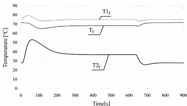
**Fig. 8.** Course of temperature changes versus time within the fresh-water cooling system (FWI) for a signal given from the ship motion system and the conditions : sea-water temperature of 10 deg C sea-water temperature control system under operation
