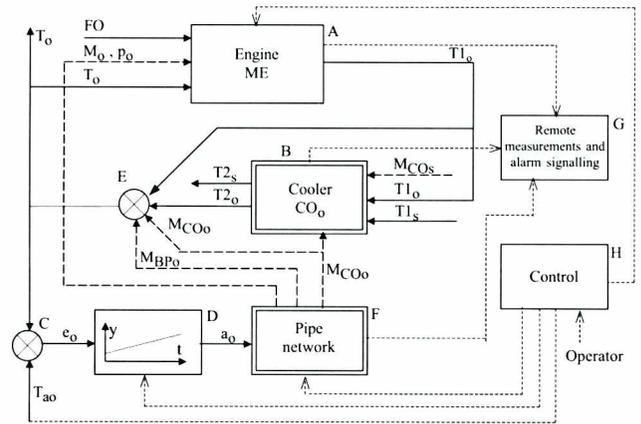
Fig.6. Model scheme of the lubricating oil cooling system of the main engine
