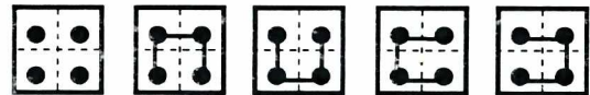
Fig.6. Possible 4-vertex configurations in 2x2 matrix and all routing solutions for these configurations
