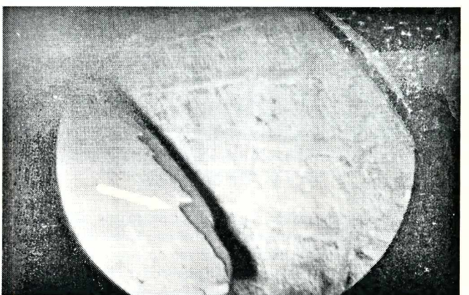
Fig.11. The rotor blade of HPT of DR77 engine. Damage (cavities) of protection coating at the blade tip edge
