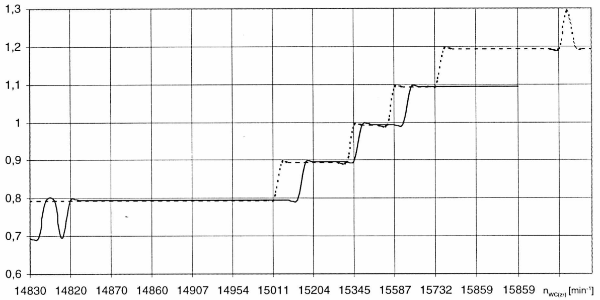
Fig. 9. Air pressure changes behind NC compressor in function of WC rotor speed
