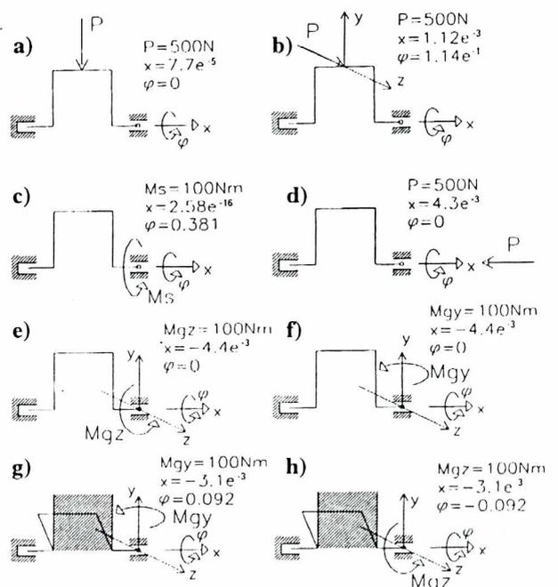
Fig.2. Deformations of a single crank under different loading (displacement  $x$  - [m], angle  $\varphi$  - [rad])
