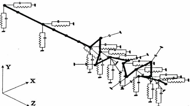
Fig.4. Simplified calculation model of the ship propulsion system in which the crankshaft is idealized by the superelements which couple the torsional and axial vibration
