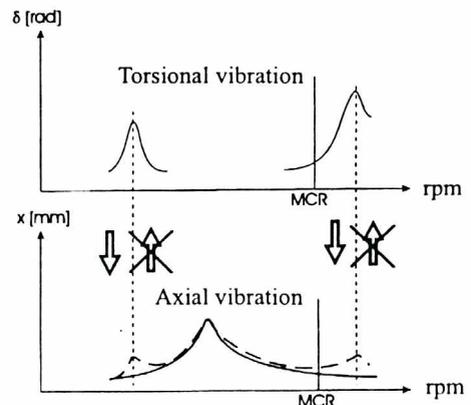
Fig.1. Scheme of mutual interaction of torsional and axial vibration
