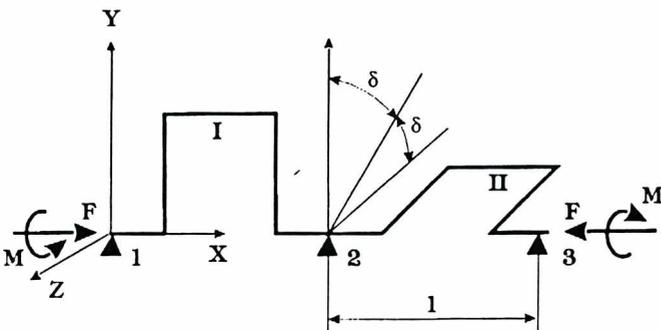
Fig.3. System of two cranks under the axial force  $F$  and torsional moment  $M$
