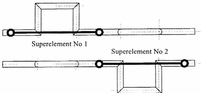
Fig.5. A crankshaft fragment modelled by two superelements of 12 d.o.f. each
