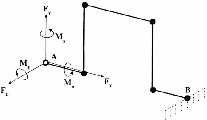
Fig.6. Model of the one-end-fixed crank used to determine the crank flexibility coefficients
