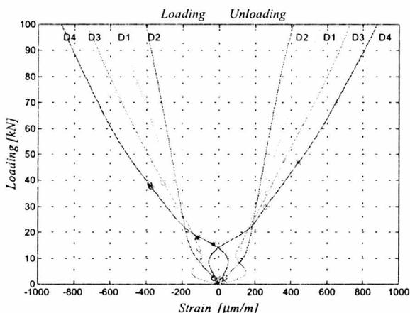
Fig.5. The dynamometers' loading measured during shafting alignment (D1, D2, D3, D4 - dynamometer numbers)
