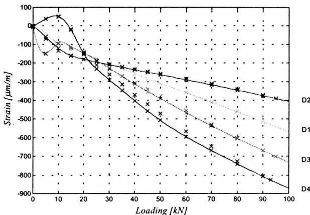
Fig. 3. Set of the dynamometer characteristics obtained at the amplification 5 of the strain - gauge bridge (D1, D2, D3, D4 - dynamometer numbers)
