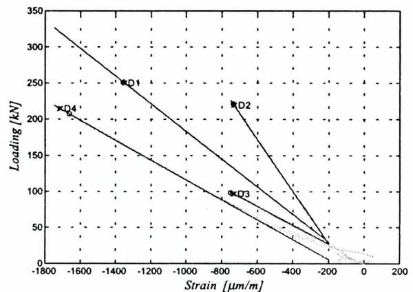
Fig.6. The dynamometers' loading measured while tensioning the foundation bolts (D1, D2, D3, D4 - dynamometer numbers)
