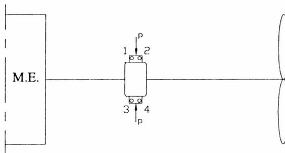
Fig. 4. The location scheme of the dynamometers and their numbering
