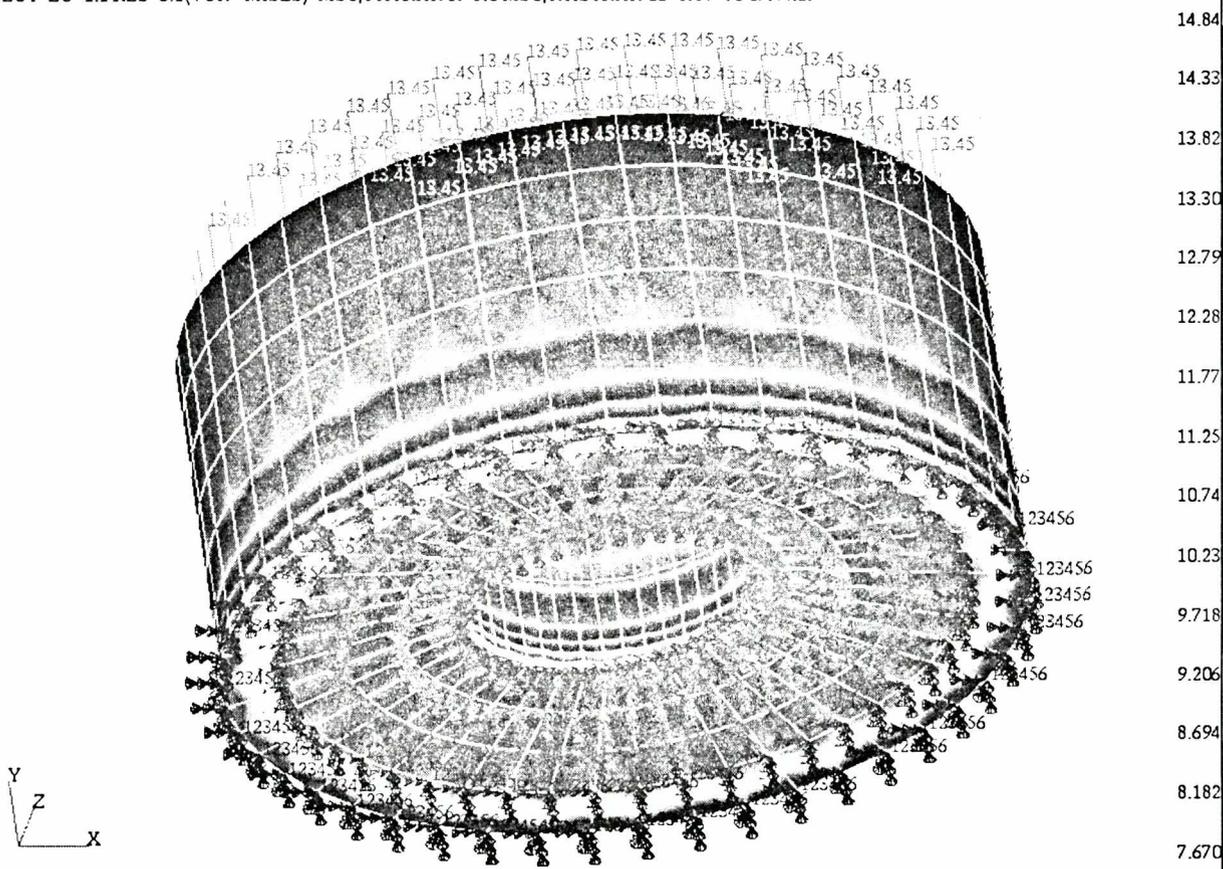
Fig. 2. Huber-von Mises stress distribution in the pad supported on its entire spherical surface
