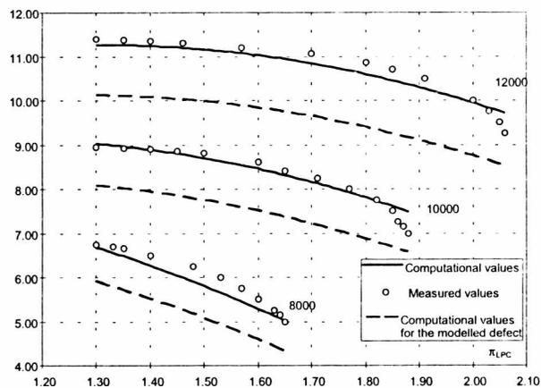
Fig. 4. LP compressor characteristics:  $m_{LPc} = f(n_{LP}, \pi_{LPc})$
