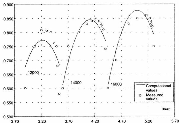
Fig. 5. HP compressor characteristics:  $\eta_c = f(n_{HP}, m_{HPc})$
