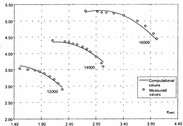
Fig. 6. HP compressor characteristics:  $m_{HPc} = f(n_{HP}, \pi_{HPc})$
