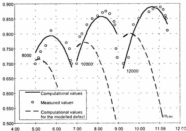
Fig. 3. LP compressor characteristics:  $\eta_c = f(n_{LP}, m_{LPc})$
