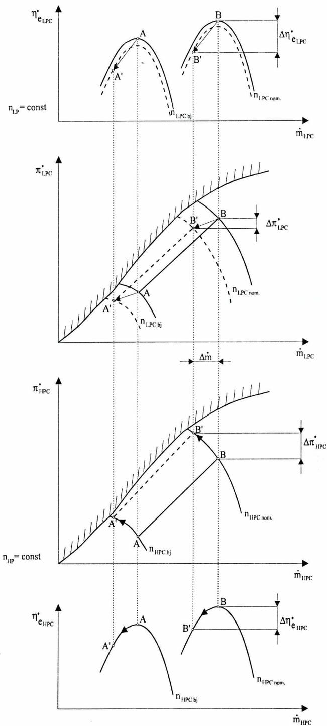
Fig.7. Shift of operating points of the LP and HP compressors in a two-shaft engine with a free power turbine caused by fouling of LP compressor inter-blade channels:
