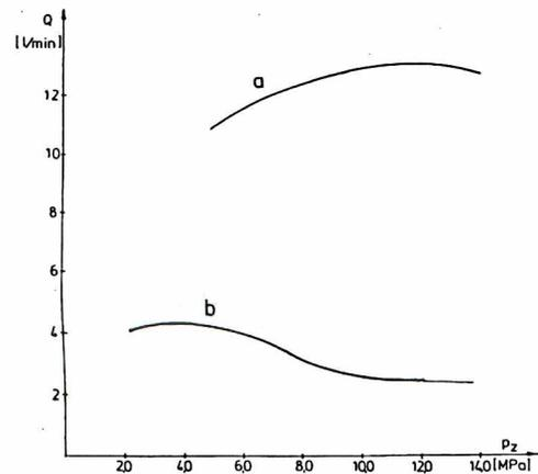
Fig. 11. Flow rate of the oil leaking out of the seal with the thick-walled sleeve *a* and that with the thin-walled sleeve *b*
