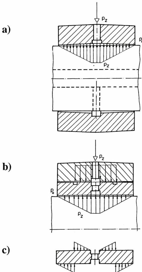
Fig. 3. Unloading principle applicable to radial seals
