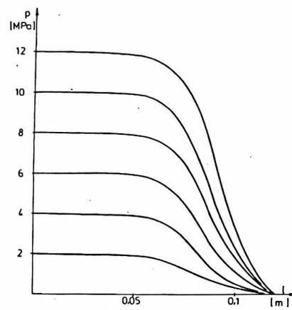
Fig. 10. Oil pressure distribution within the bearing interspace of the seal with the thin-walled sleeve *b*
