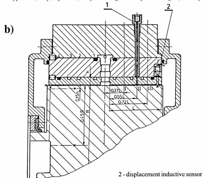
Fig. 8. Axial cross-section through the investigated seal with the sleeve b
