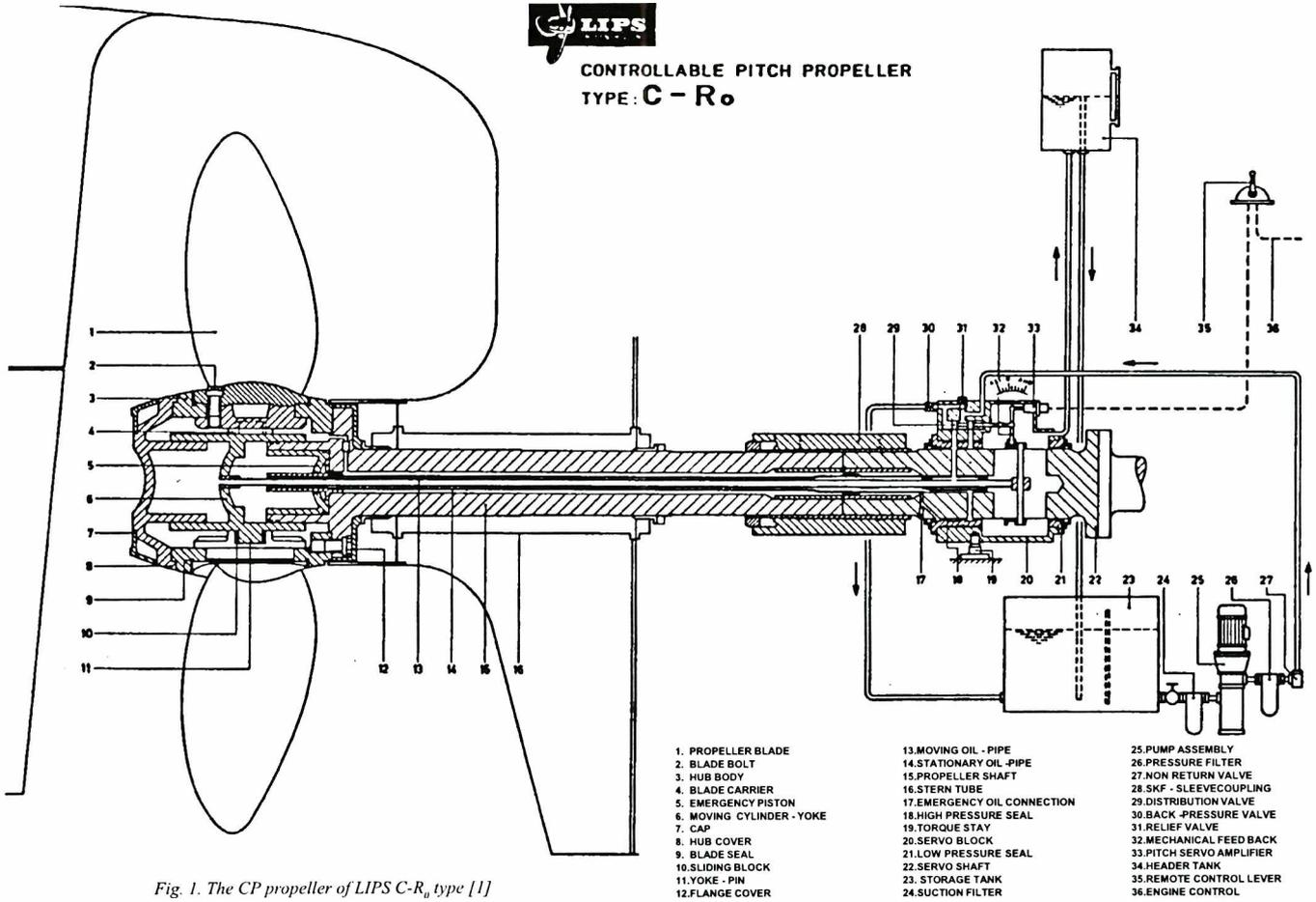
Fig. 1. The CP propeller of LIPS C-R<sub>0</sub> type [1]
