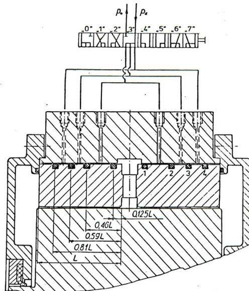
Fig. 5. Realization scheme of eight different unloading levels in the tested seal
