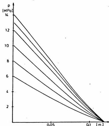
Fig. 9. Oil pressure distribution within the bearing interspace of the seal with the thick-walled sleeve *a*
