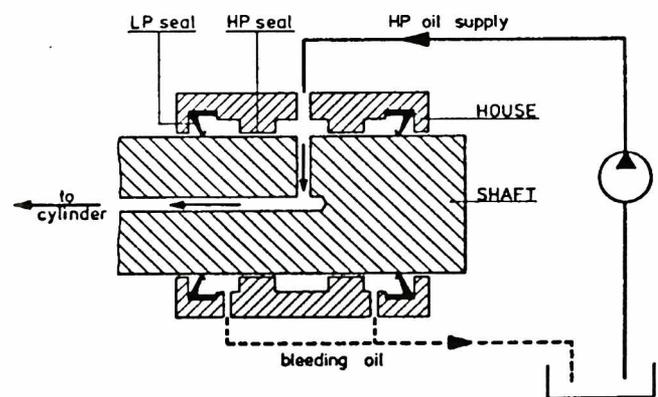
Fig. 2. The radial seal used in the CPP low-pressure installations
