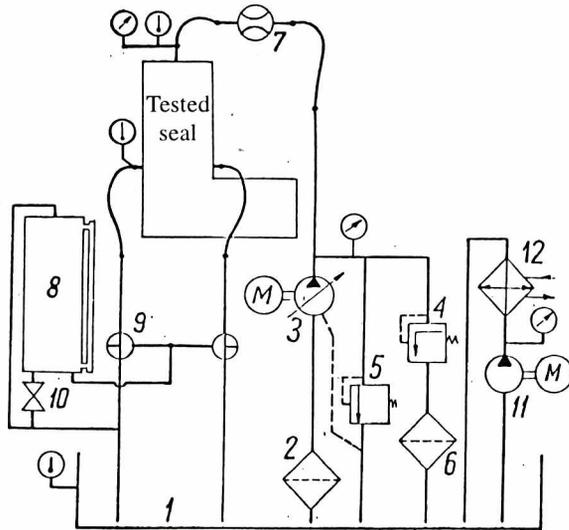
Fig. 6. Hydraulic supply unit scheme
