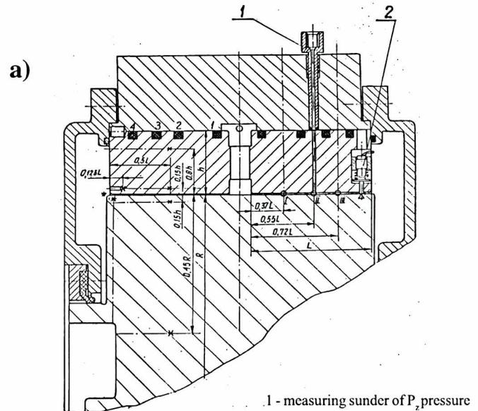
Fig. 7. Axial cross-section through the investigated seal with the sleeve a
