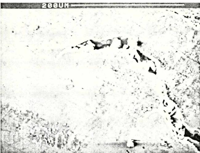
Fig. 4. Surface hydrogen crack on AlZn5Mg1 alloy ( $tb_{22}$ ) alloy specimen after stress corrosion exposure under the applied potential of -200 mV in relation to  $U_{st}$ ,  $t = 1000$  h, 274 x enlarged, SEM.
