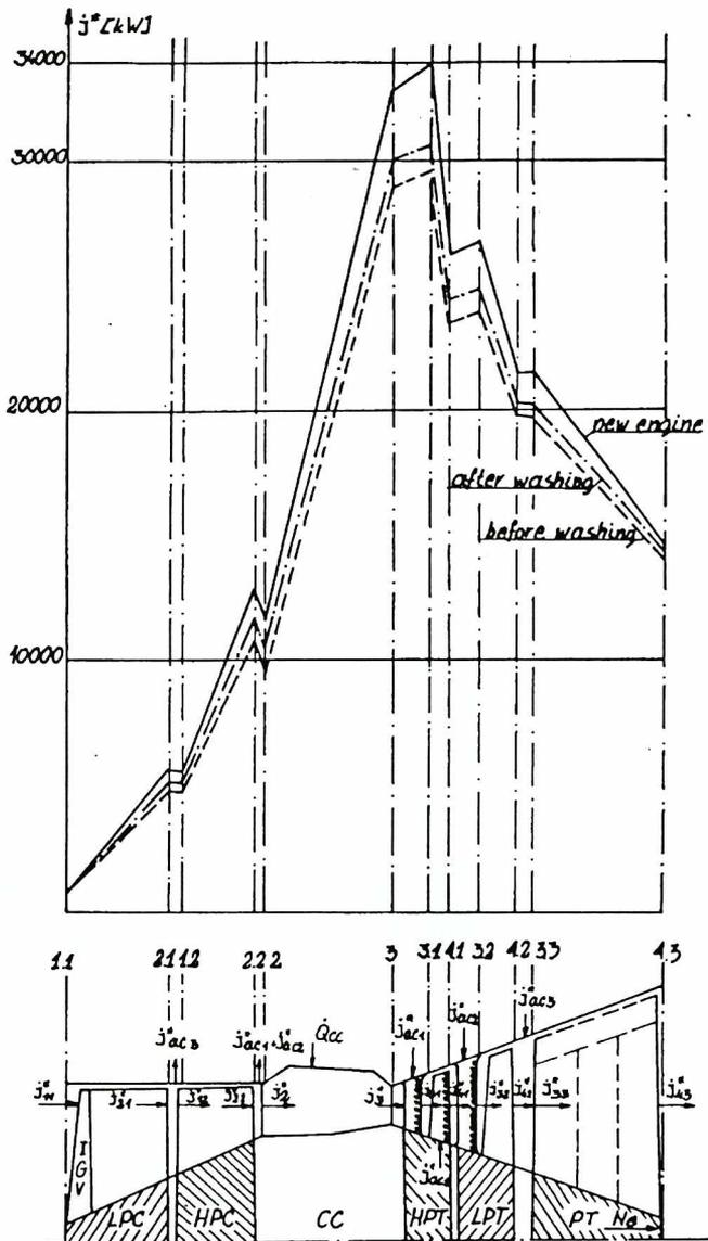
Fig. 10 Distribution of enthalpy flux in control sections of the engine
