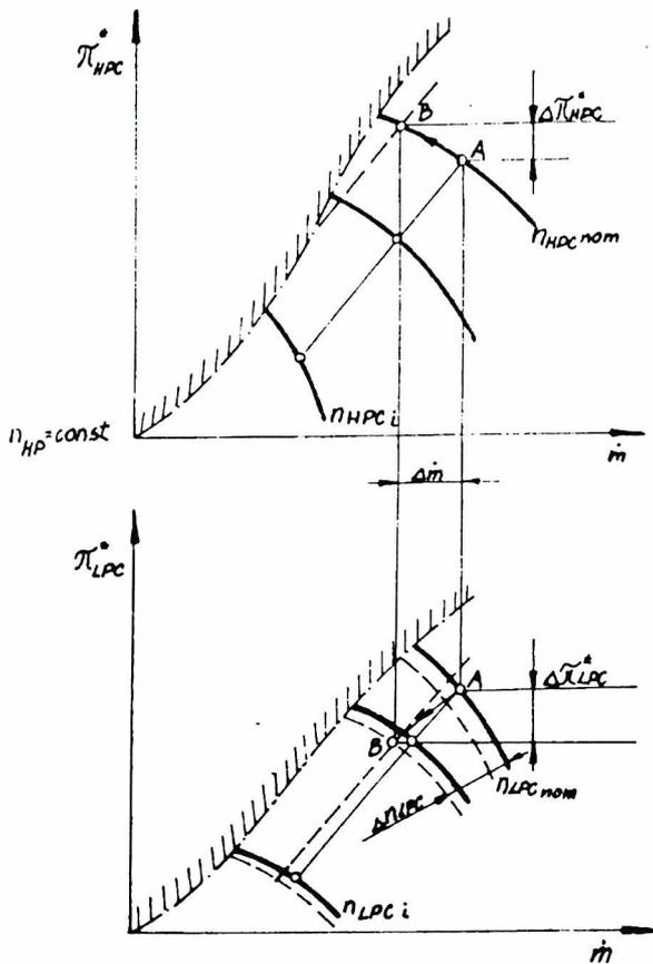
Fig. 2 Shift of operating points of the LP and HP compressors in a two-shaft engine with a free power turbine caused by fouling of LP compressor blade channels
