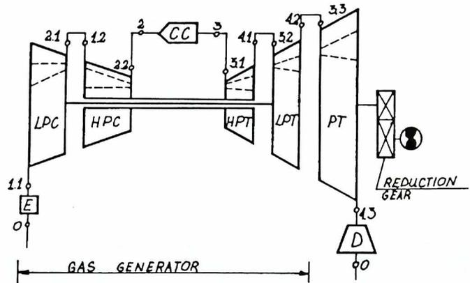
Fig. 3 Schematic diagram of a two-shaft engine with a free power turbine: E - intake dust extractor, D - exhaust diffuser manifold, LPC - low pressure compressor, HPC - high pressure compressor, HPT - high pressure turbine, LPT - low pressure turbine, PT - power turbine, CC - combustor
