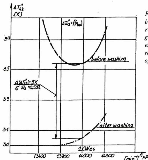
Fig. 7 Relation between temperature rise of gas generator exhaust and the rotational speed of the HP shaft
