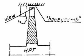
Fig. 9 The enlarged radial clearance of the HP turbine shaft resulting of its seizure
