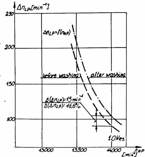
Fig. 8 Changes of differences between rotational speeds of the LP and HP shafts as a function of the HP shaft speed
