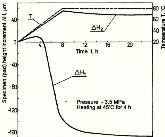
Fig. 3. Creep curves for the specimens and pad of the EPY plastic.
