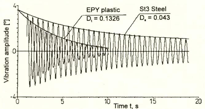
Fig. 5 Vibration amplitude-time response characteristics for the EPY plastic and the St3 steel at 20°C.
