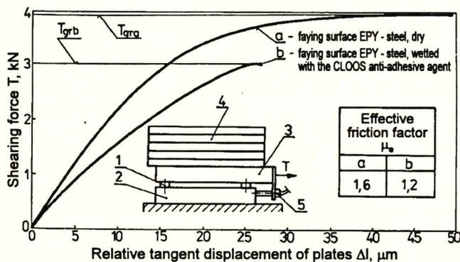
Fig. 4. Curves illustrating relationship of the shearing force  $T$  to the relative tangent displacement along the faying surfaces between the EPY plastic and steel. 1 - elements cast of the EPY plastic, 2 & 3 - steel plates, 4 - weight pads, 5 - displacement gauges.
