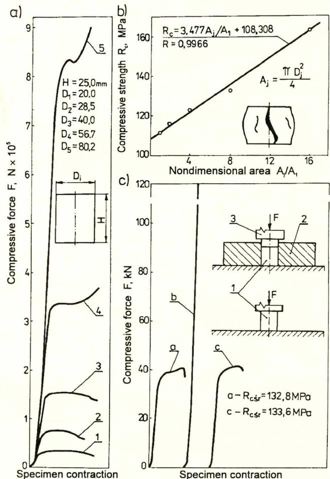
Fig. 2. Compressive test diagrams for the EPY plastic (a, c), and compressive strength-size relation for the plastic specimens (b).
