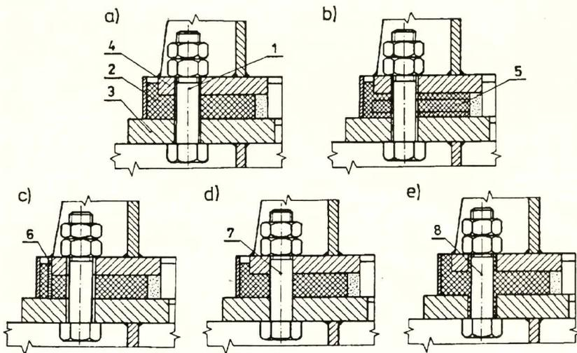
Fig. 1. The standard foundation bolted joint with the pad cast of EPY plastic (a) and its version (b, c, d, e).
