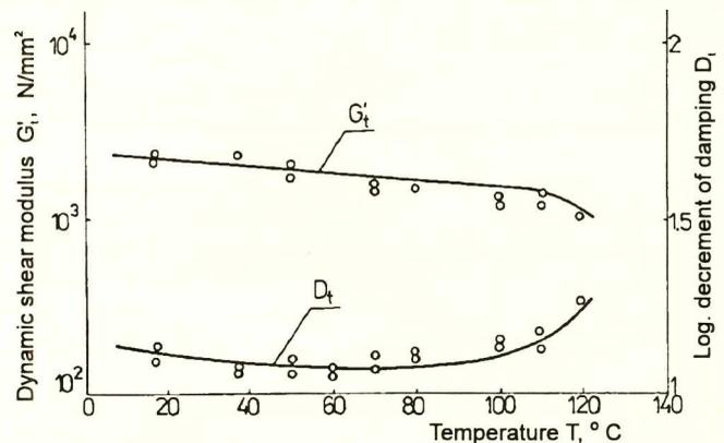
Fig. 6 Relationship of the logarithmic decrement of damping  $D$  and dynamic shear modulus  $G'$  to temperature for the EPY plastic.
