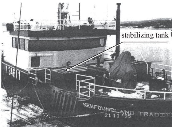
Rys. 4. Stabilizing tank in the form of container installed on deck of a fishing ship [2]
