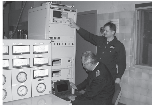
Diesel engine test stand equipped with MEXA 9300 Horiba exhaust gas analyzer, at Polish Naval University, Gdynia
