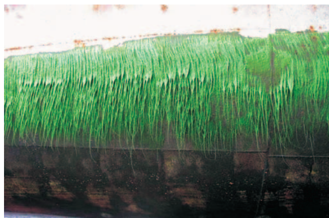
Fig. 4. Algae fouling the ship hull .
