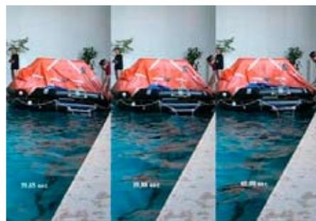
Figure 10. Checking the roll time for the life raft.
