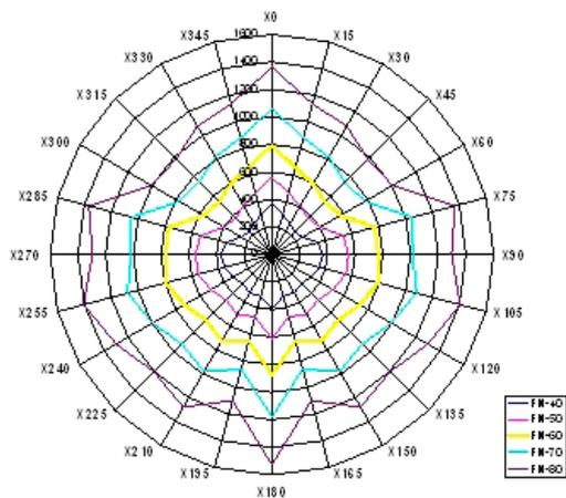
Figure 6. The space distribution of wind heeling force, steady conditions-40, 50, 60, 70, 80 kn wind speed, results from wind test tunnel for a ten-person life raft, [7].
