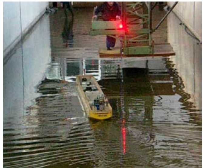
Figure 5. Model during the evasive manoeuvre test
