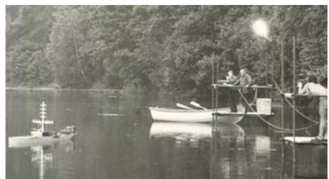
Figure 8 Model during the turning test, joniny station, in the second half of the seventies
