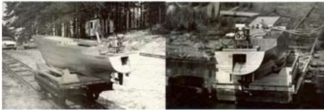
Figure 9 Model of the ship (m/s "Profesor Siedlecki") positioned on the launching carriage
