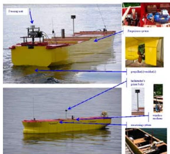
Figure 5 Equipment used during free sailing manoeuvring model tests at the present time
