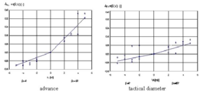
Fig. 6. Dependence of advance and tactical diameter values on the wind angle and velocity
