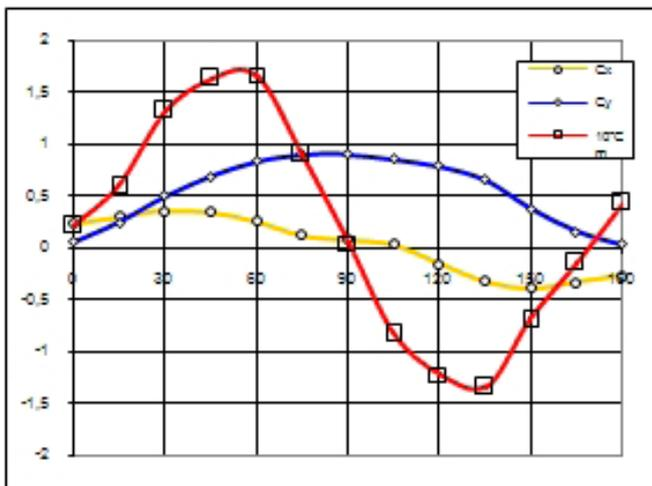
Fig. 2B Aerodynamic characteristics of ship model M467 with the wind simulation system [3]
