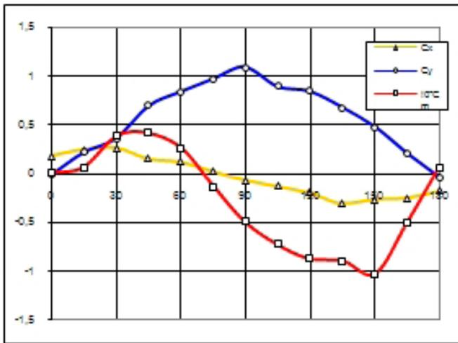
Fig. 2A Aerodynamic characteristics of ship model M509 [2]
