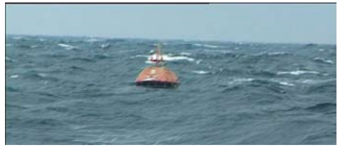
Fig. 8 10-person life raft during the tests conducted in real sea conditions.
