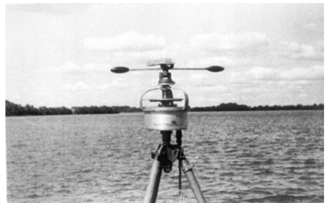
Fig. 5. Parent selsyn transmitting angle information – first version without telescopes
