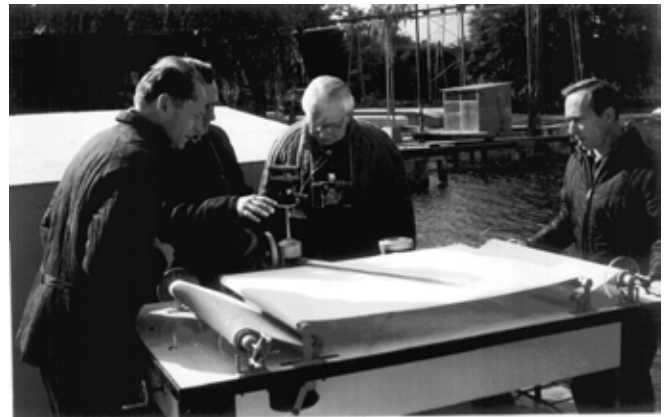
Fig. 4. Improved version of torograph with optical telescopes and trace burning
