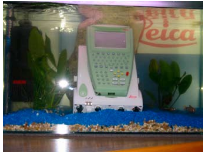
Fig. 10. New Leica GX1230 GPS during an underwater test
