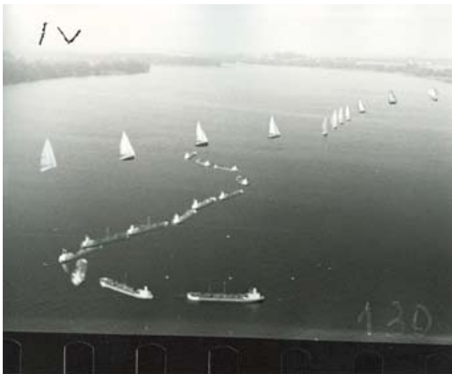
Fig.1. Frame-by-frame photographs of a 105,000 DWT OBO ship model trajectory. Mix of 13 frames.
