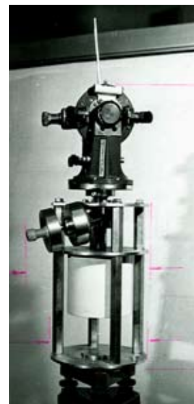
Fig. 6. Model tracking point with an optical telescope and angle transducer
