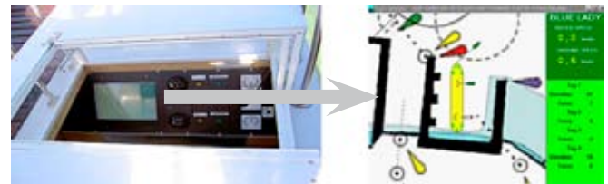
Fig. 12 - Control panel of a tug simulator and a monitor screen with transitory tug positions
