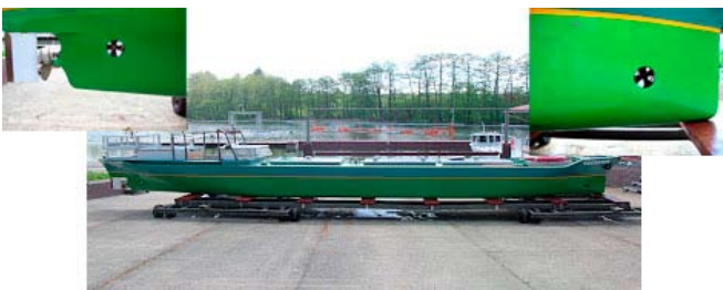
Fig. 11 - Training model „Szczecin” equipped with a bow thruster and stern thruster. They had a tug operation simulation option
