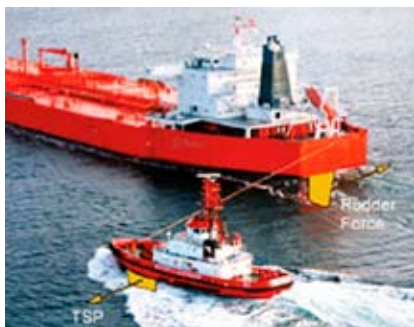
Fig. 7 - Tug in escorting operation. The marked ship steering force is generated by the tug skeg
