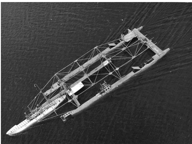
Figure 4. Modified floating measurement platform
