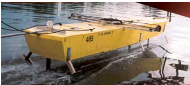
Fig. 15. Model of a single-hull hydrofoil with a set of three foils under tests on Jeziorak Lake
