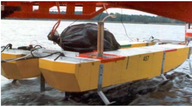
Fig. 13. Model of catamaran, supported by a set of three foils, under tests
