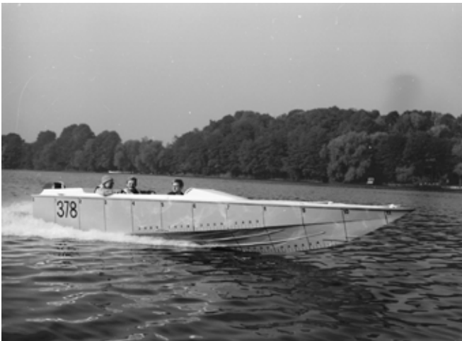
Fig. 20. Self-propelled model in 1:5 scale on Jeziorak Lake
