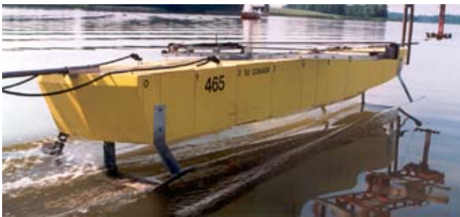
Fig. 14. Model of a single-hull hydrofoil with a set of two foils under tests on Jeziorak Lake
