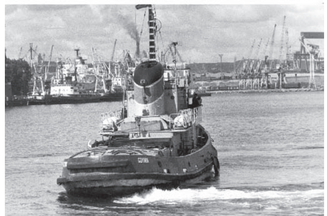
Fig. 4. Photo of Tug "Achilles" showing her manoeuvring ability and producing transverse force.
