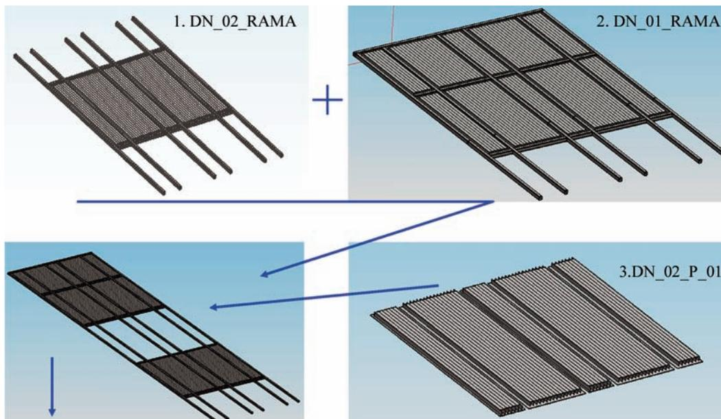
Fig. 4. Bottom region prefabrication.
