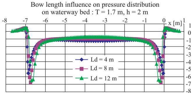
Fig. 7. Bow length influence on pressure distribution on waterway bed, for B\_89 form.
