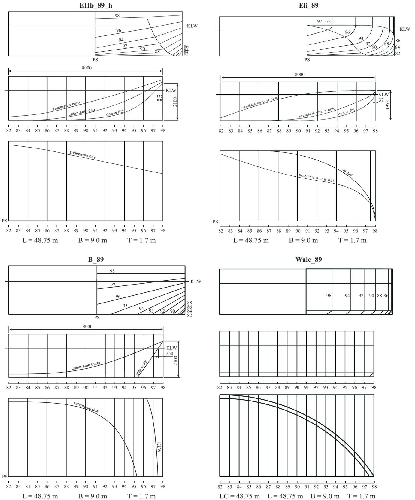
Fig. 2. Barge hull forms assumed for the analysis .
