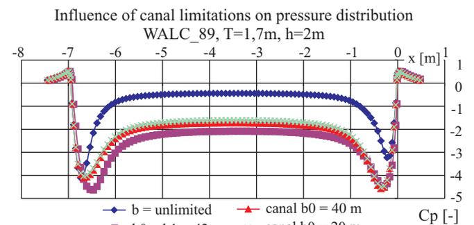
Fig. 6. Influence of canal limitations on pressure distribution on waterway bed, in ship's plane of symmetry .
