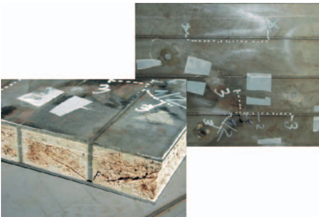
Fig. 3. Fatigue cracks in the model .
