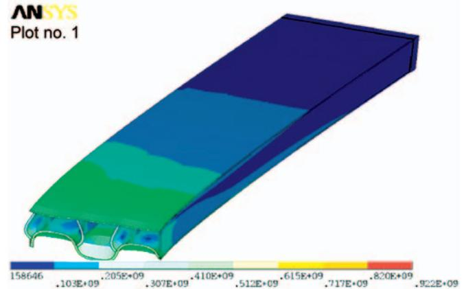
Fig. 6. Stress distribution in shell plating and stiffeners .
