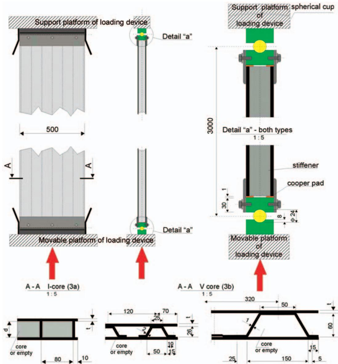
Fig. 2. In-plane load geometry and loading scheme of the tested models.
