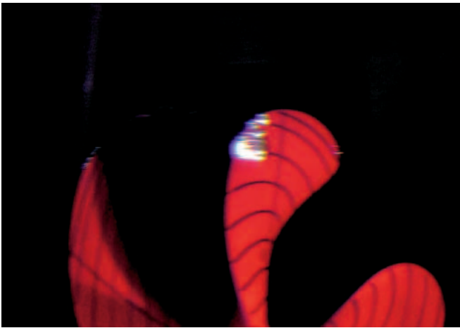
Fig.2. Cavitating tip vortex approaching rudder – phase 2.
