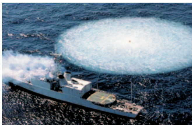
Fig. 3. Experimental tests of shock strength of frigates against underwater explosion.
