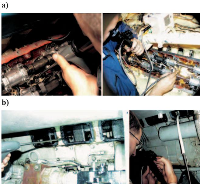
**Fig. 6.** Ways of inserting the end of borescope and fiberscope into cylinder interior of: **a)** M401A-1 diesel engine – through the holes remaining from dismantled injectors, **b)** 16V149TI Detroit Diesel engine – through inlet air windows in cylinder liner.
